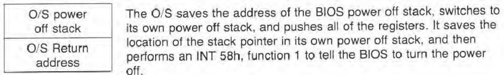
4. When the power is turned back on, and the BIOS determines that a Warm Start Break is to be performed, it transfers control to the O/S entry point with AL = 2 to indicate that a Warm Start Break should occur.
