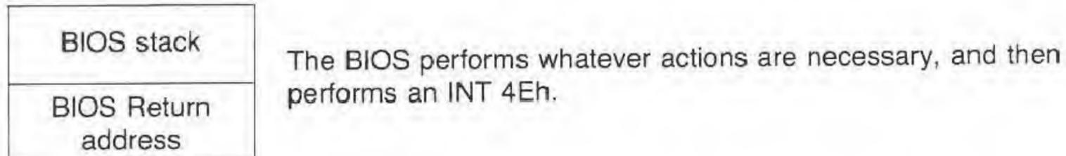
3. The INT 4Eh transfers control to the O/S Power Off Hook, which saves the machine state so that it can be restored during Warm Start Resume.
