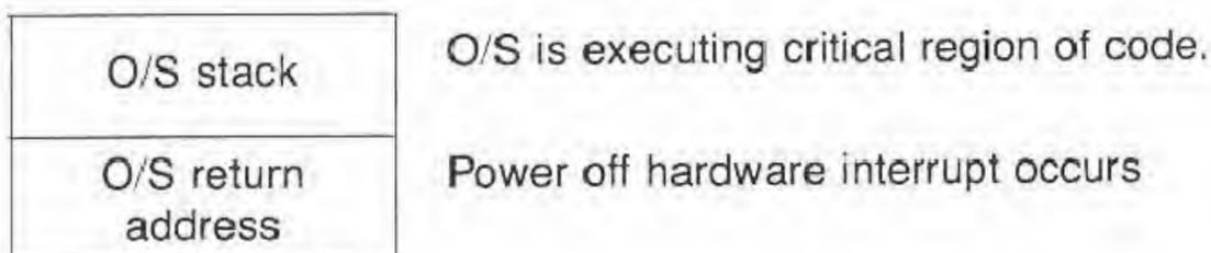
2. The hardware interrupt transfers control to the BIOS, which switches to its own interrupt handler stack.
