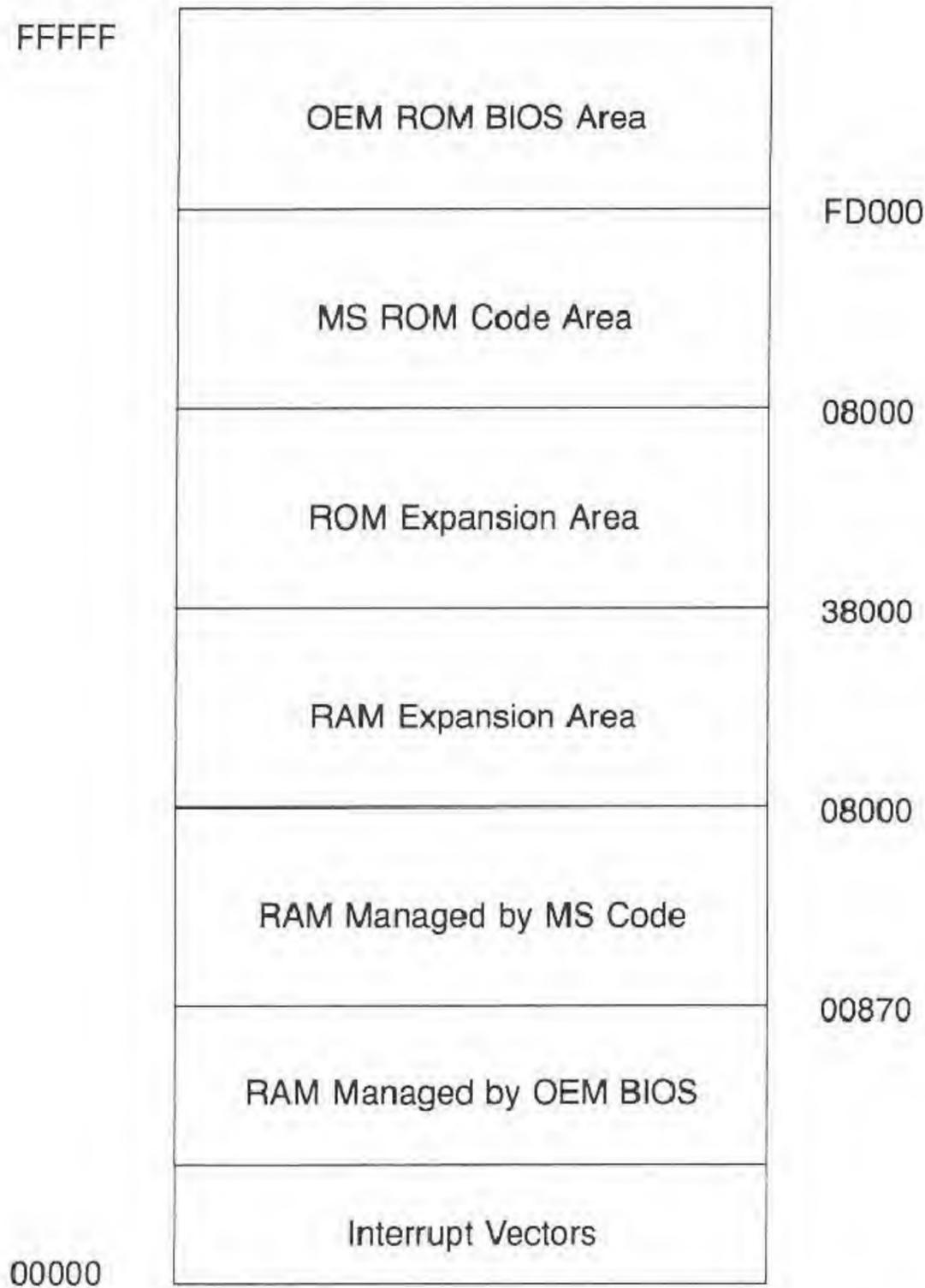
The interrupt vectors in the range 40h - 4Fh are reserved for use by the Microsoft ROM code, any interrupts outside of this range may be used by the OEM.
